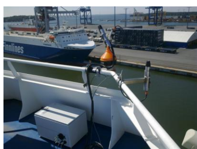
Figure 2-1: Rflex platform with hyperspectral Rrs instrument installed on M/S Finnmaid (Finnlines)
